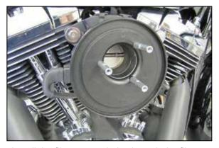
7. Install the filter spacer bolts through the filter back plate and then install the gasket onto the spacer bolts passed through the back plate. Install the filter back plate assembly onto the breather plate and secure with the filter spacer bolts. NOTE: Be sure to place one drop of thread locker on each bolt.
