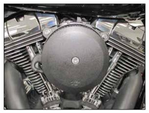
10. Install the filter cover plate onto the filter and secure with the provided hardware.
