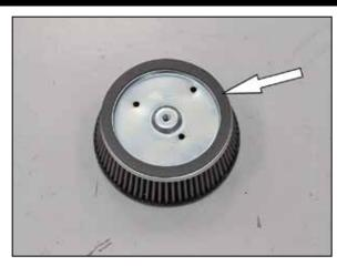
8. Install the provided gasket onto the filter top plate as shown.
