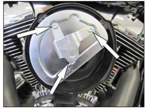
3. Remove the three bolts which secure the air filter to the filter base and then remove the air filter along with the crank case breather tube and bonnet bracket.
