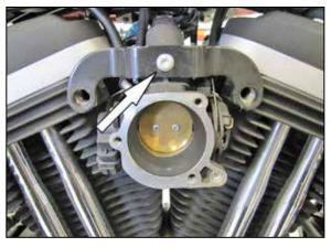
5. Remove the bolt securing the throttle body bracket and then remove the throttle body bracket from the vehicle.
