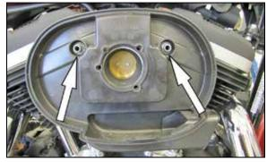
4. Remove the O-Rings from the breather bolts and then remove the breather bolts and rear air filter
