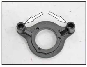
6. Install two of the provided O-Rings into the K&N® throttle body bracket as shown.
