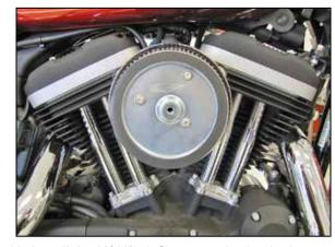
10. Install the K&N® air filter onto the back plate and secure with the provided hardware. NOTE: Be sure to place one drop of the provided thread locker onto the threads of the bolts.
