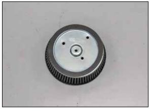
9. Install the provided gasket onto the K&N<sup>®</sup> air filter as shown.
