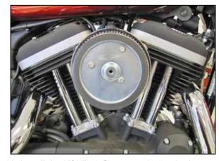
10. Install the K&N® air filter onto the back plate and secure with the provided hardware.
