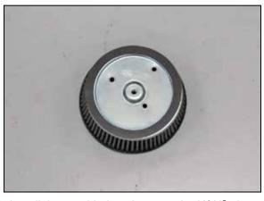
9. Install the provided gasket onto the K&N<sup>®</sup> air filter as shown.
