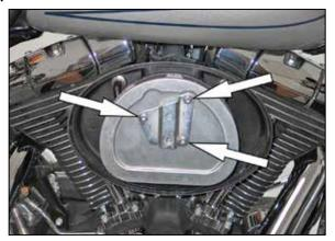
3. Remove the three bolts that secure the air filter to the filter base and then remove the air filter along with the crankcase breather tubes. **NOTE: The factory air filter may differ from the picture; it may also have a bracket attached.**
