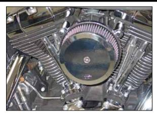
12. Install the filter cover plate onto the K&N<sup>®</sup> air filter and secure with the provided hardware. **NOTE: Be sure to place one drop of thread locker to the cover plate mounting bolt.**
