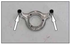
7. Install two of the provided o-rings into the K&N $^{\otimes}$  crankcase breather plate as shown.
