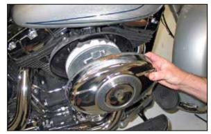
2. Remove the bolt that secures the bonnet to the
