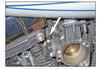
6. Using the provided tie wrap, secure the wiring pig tail to the throttle body wiring harness. **NOTE: On non-US models, a by-pass module**
