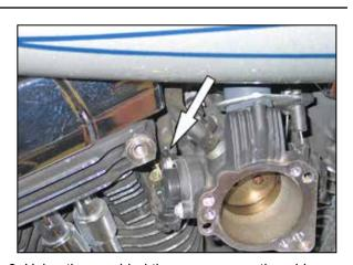
6. Using the provided tie wrap, secure the wiring pig tail to the throttle body wiring harness. NOTE: On non-US models, a by-pass module
