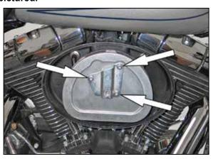
3. Remove the three bolts that secure the air filter to the filter base and then remove the air filter along with the crankcase breather tubes. NOTE: The factory air filter may differ from the picture; it may also have a bracket attached.
