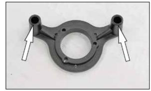
7. Install two of the provided o-rings into the K&N® crankcase breather plate as shown.
