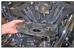
5. Remove the air filter base from the throttle body and unhook the wiring pig tail from the filter base. NOTE: Some models do not have the wiring pigtail.
