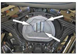
3. Remove the three bolts which secure the air filter to the filter base and then remove the air filter along with the crank case breather tubes. NOTE: The factory air filter may differ from the
