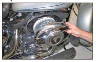
2. Remove the bolt which secures the bonnet to the filter assembly and then remove the bonnet from
