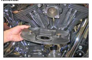
5. Remove the air filter base from the throttle body and unhook the wiring pig tail from the filter base. NOTE: Some models do not have the wiring pigtail.
