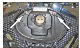
4. Remove the two crank case breather bolts
