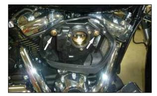
2. Remove air filter cover bolt and air filter cover as shown.
