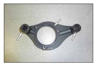
7. Install three of the o rings provided onto the back side of the K&N<sup>®</sup> back plate as shown. A small amount of grease maybe used to hold the o rings in place.
