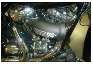
11. Install the K&N<sup>®</sup> intake tube with the gasket and provided hardware.
