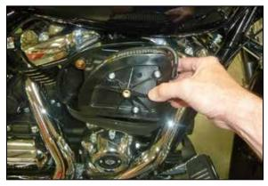
4. Remove the air filter from the vehicle and disconnect the crankcase breather tubes.
