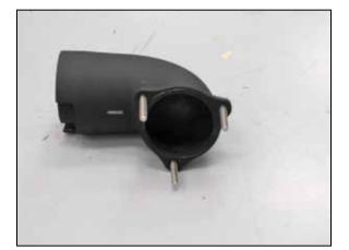
9. Install the provided O-ring and tube mounting bolts into the intake tube as shown.
