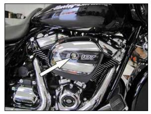
2. Loosen and remove the bolt which secures the decorative filter cover and remove the cover from the vehicle.
