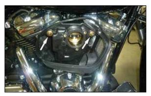
5. Remove the two breather/air filter base mounting bolts as shown.
