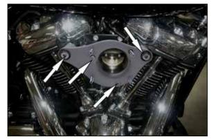
10. Using the two provided crankcase breather bolts; install the back plate onto the vehicle. Do not tighten bolts at this time. Then secure with the two other bolts provided. Tighten all bolts at this time. NOTE: Apply one drop of the provided thread locker onto the bolts.
