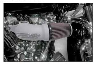
12. Install the K&N $^{\!0}$  air filter onto the intake tube and secure with the provided hose clamp.
