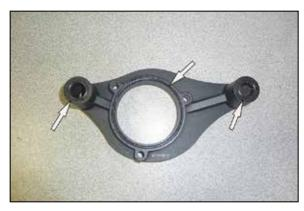
7. Install three of the o rings provided onto the back side of the K&N® back plate as shown. A small amount of grease maybe used to hold the o rings in place.
