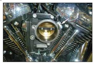
9. Install the long stud as shown  $\frac{1}{2}$ " down. Note; apply one drop of thread locker onto stud.
