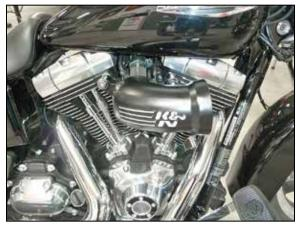
11. Install the K&N® intake tube with the gasket and provided hardware.
