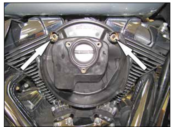
5. Remove the two factory crank case breather bolts and then remove the filter back plate from the vehicle.
