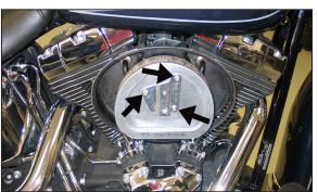
3. Remove the three air filter retaining bolts shown.
