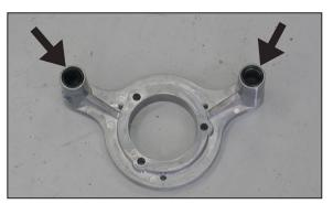
8. Install two of the o rings provided onto the back side of the  $K\&N^{\otimes}$  back plate as shown.
