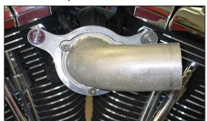
12. Install the K&N® intake tube with the gasket and secure with the provided hardware.
