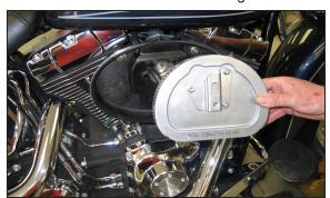
4. Remove the air filter with the breather hoses as shown.
