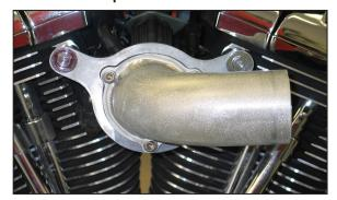
12. Install the K&N® intake tube with the gasket and secure with the provided hardware.
