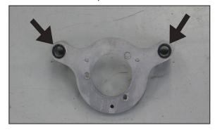
9. Install the remaining two provided o rings onto the front of the back plate as shown.
