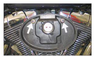
5. Remove the two crankcase breather bolts shown.
