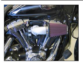
10. Install the provided K&N<sup>®</sup> air filter and secure with the provided hose clamp. A black hose clamp is being supplied with kit. This clamp is intended to clamp the filter to the intake tube. **NOTE: Drycharger<sup>®</sup> air ilter wrap; Part # RC3680DK is available to purchase separately.**  11. Double check to make sure everything is tight and properly positioned before starting the vehicle.
