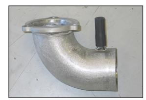
8. Trim the provided crankcase breather hose to a length of 1.5" and then install it onto the K&N® intake tube as shown.
