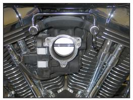
7. Install the supplied crankcase breather tube using the provided breather bolts and washers. NOTE: Place one washer on each side of the of the breather tube.
