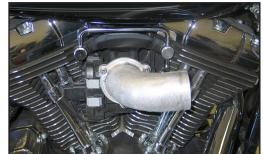
3. Loosen the three air filter retaining bolts shown.
