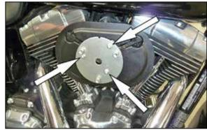
5. Remove the three retaining bolts for the air filter adapter as shown.
