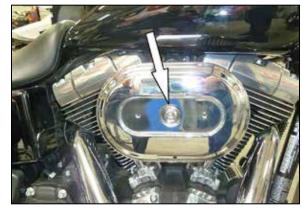
3. Remove the air filter cover retaining bolt and remove the air filter cover.
