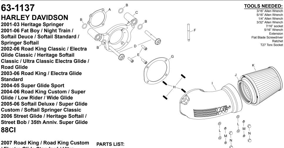
B O-Ring; 9/16" ID, .10 Thick С Back Plate; Harley 1 63-1137-2 Hose Clamp #48 08601 D Breather Bolt 2 22237 Air Filter RE-5286 E Screw: 1/4-20 x 3/4" SOC. 07731 Washer: Flat #10 SS 08257 Thread Locker 482 Washer; Lock #10 SS 22241 G Gasket; 63-1134 63-1134-3 10-32 Cap Nut 22239
