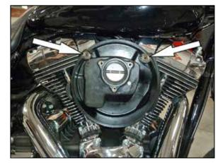
6. Remove the two breather/air filter base mounting bolts as shown.
