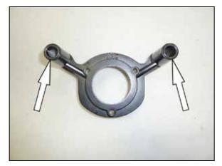
8. Install two of the o rings provided onto the back side of the K&N<sup>®</sup> back plate as shown.
