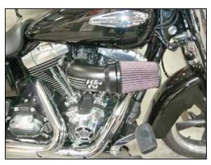
12. Install the K&N<sup>®</sup> air filter onto the intake tube and secure with the provided hose clamp.
