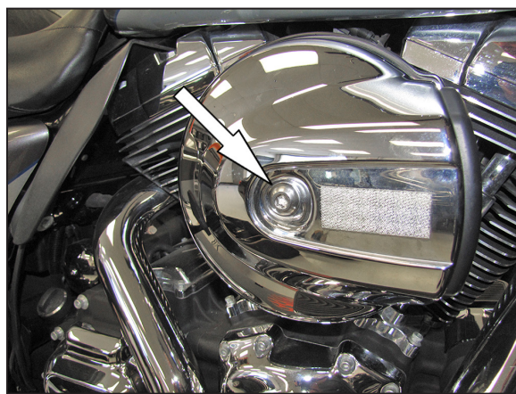
3. Remove the bolt securing the air filter cover and then remove the cover from the vehicle.
