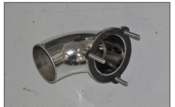
6. Install the three provided tube mounting bolts into the K&N® intake tube and then install one of the two provided gaskets onto the bolts.
