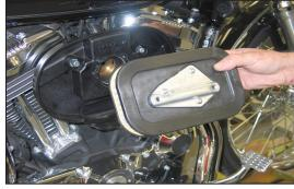
4. Remove the air filter as shown.
