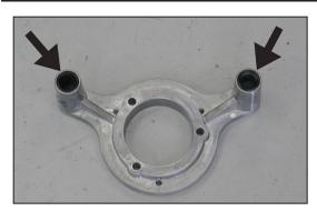
8. Install two of the o rings provided onto the back side of the K&N® back plate as shown.
