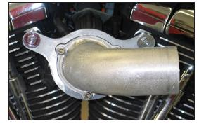
12. Install the K&N $^{\odot}$  intake tube with the gasket and secure with the provided hardware.
