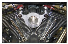
10. Using the two provided crankcase breather bolts; install the back plate onto the vehicle as shown. Do not tighten the breather bolts at this time.
