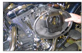
6. Remove the air filter breather base as shown. NOTE: K&N Engineering, Inc. recommends that customers do not discard the factory air intake components.
