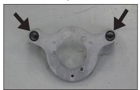
9. Install the remaining two provided o rings onto the front of the back plate as shown.
