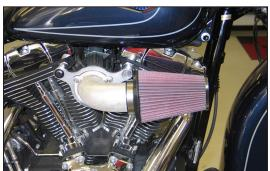
13. Install the K&N® air filter onto the intake tube and secure with the provided hose clamp. A black hose clamp is being supplied with kit. This clamp is intended to clamp the filter to the intake tube.
