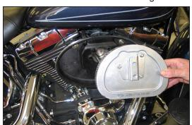
4. Remove the air filter with the breather hoses as shown.
