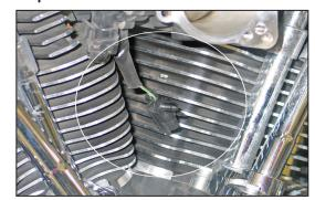
7. Using the provided tie wrap, secure the loose pig tail to the to the throttle position switch wiring harness
