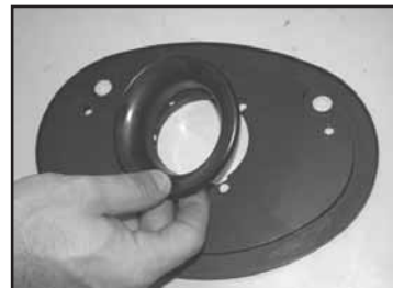
9. Reinstall the velocity stack onto the back plate.
