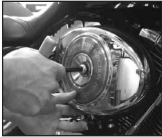
1. Remove the air cleaner cover.
