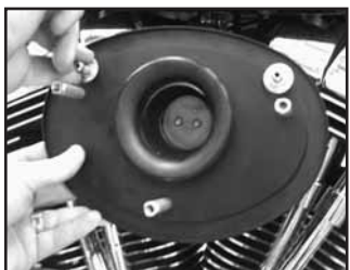
5. Remove the two stock breather bolts.
