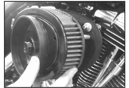
16. Install the K&N® air filter onto the base plate.
