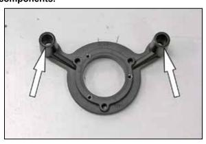
5. Install two of the provided O-rings into the crank case breather plate as shown.
