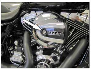
2. Remove the bolt which secures the bonnet to the filter assembly and then remove the bonnet from the vehicle.
