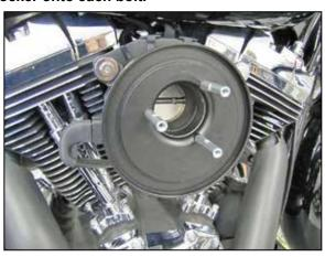
7. Install the filter spacer bolts through the filter back plate and then install the gasket onto the spacer bolts passed through the back plate. Install the filter back plate assembly onto the breather plate and secure with the filter spacer bolts.
