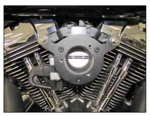
6. Install the crank case breather plate along with the two remaining O-rings, breather bolts, throttle body mounting bolts and throttle body gasket as shown
