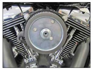
9. Install the filter onto the base plate and secure with the provided hardware.
