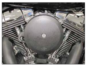
10. Install the filter cover plate onto the filter and secure with the provided hardware.
