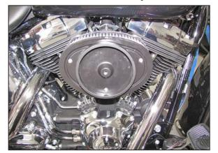
11. Install the K&N<sup>®</sup> air filter and secure with the
