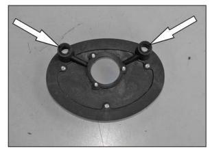
9. Install the two provided O-Rings onto the crank case breather ports.
