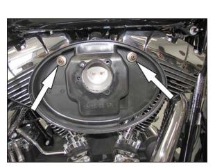
4. Remove the stock breather bolts which secure the stock air filter base shown.
