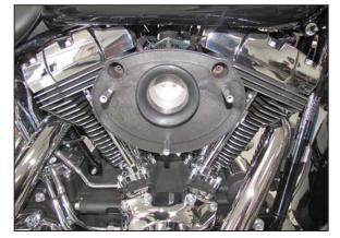
10. Install the back plate and secure with the stock breather bolts. Tighten the three bolts that secure the back plate to the throttle body. Then tighten the two breather bolts fully.
