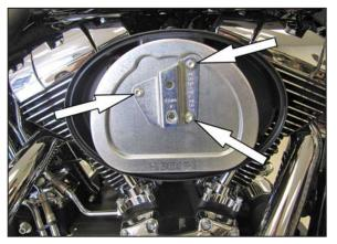
3. Remove the three bolts which secure the stock air filter element. Then remove the stock air filter element and stock crank case breather hoses as shown.
