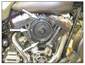
13. Install the K&N<sup>®</sup> air filter onto the back plate and secure with the provided hardware. **NOTE: Place one drop of thread locker onto the bolts before installing.**
