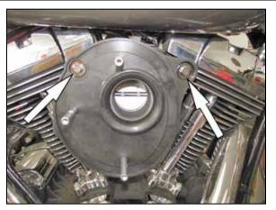
12. Place one drop of thread locker onto the breather bolts and then install the breather bolts into the back plate as shown.
