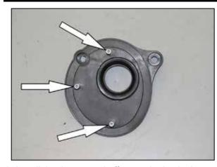
8. Install the three stand-offs onto the back plate using the provided hardware. **NOTE: Place one drop of the supplied thread locker onto the threads of each bolt.**
