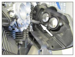
4. Pull the filter base away from the throttle body then release the spring clamp securing the crank case vent hose and disconnect the crank case vent hose from the back plate.
