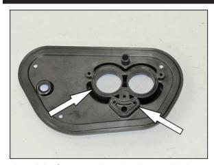
8. Install the factory gaskets into the provided K&N® back plate as shown.
