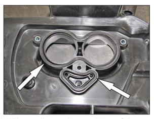
6. With a small screw driver or pick, carefully remove the factory gaskets from the filter back plate.
