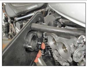
12. Attach the crank case vent hose to the K&N® pack plate.
