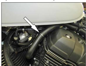
14. Cut the factory crank case vent hose in the area indicated by the line.
