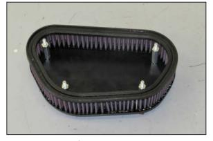
17. Install the  $K\&N^{\otimes}$  air filter onto the front plate as shown.
