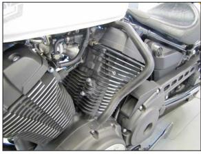
5. From the left side of the vehicle, pull the crank case vent hose out for later access.
