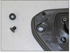
7. Remove the reinforcement and mounting grommet from the back plate as shown.
