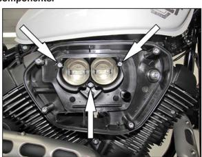
3. Remove the three Throttle body bolts and the mounting bolt shown.
