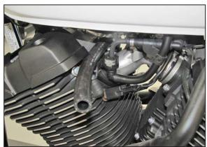
11. Route the provided crank case vent hose on top of the throttle body as shown so that it comes out of the left side of the engine.
