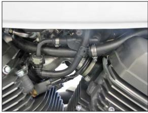
15. Trim the provided crank case vent hose for best fit, then using the provided hose mender and clamps, connect the crank case vent hoses together.
