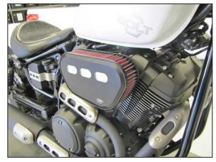
18. Install the front plate and filter assembly onto the back plate and secure to it to the back plate with the provided hardware.
