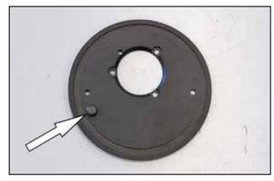
9. Install the provided rubber plug into the back plate from the back side as shown.
