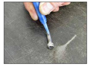
7. Apply one drop of the provided thread locker to the provided throttle body bolts.
