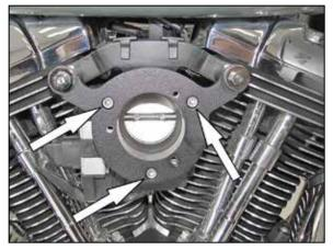
8. Install the provided throttle body gasket and then install the throttle body bolts. Secure the adapter with the two breather bolts and three throttle body bolts.
