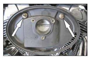
4. Remove the two breather bolts and then remove the inner air filter base.
