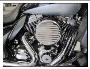
13. Install the K&N<sup>®</sup> air filter and front plate onto the back plate and secure with the provided hardware. **NOTE:** It may be helpful to use a small screwdriver to position the filter into the grooves of the front and back plate while tightening the hardware.
