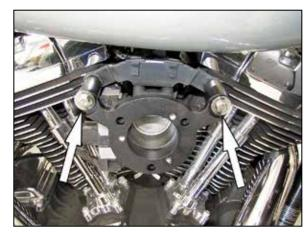
6. Install the K&N<sup>®</sup> adapter onto the engine and throttle body using the provided breather bolt. **NOTE: Do not completely tighten the breather** bolts at this time. Take care while installing the adapter so that the "O" rings do not get
