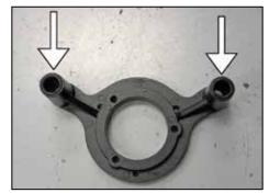
3. Remove the three bolts which secure the air filter to the filter base and then remove the <u>air filter</u> along with the crankcase breather tubes.
