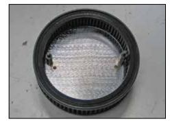
12. Install the K&N $^{\mbox{\tiny 8}}$  air filter onto the top plate as shown.
