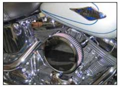
13. Install the filter/top plate assembly onto the base plate and secure with the provided hardware and thread locker.
