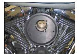
10. Install the three filter base plate mounting bolts into the base plate; install the remaining gasket and one drop of thread locker on each bolt. Secure the filter base plate to the breather plate as shown.
