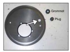
7. On vehicles equipped with a EVAP vent line, install the provided grommet into the hole shown. On vehicles not equipped with an EVAP vent line, install the provided plug into the hole shown from the back side of the base plate.
