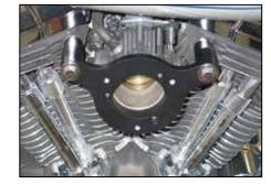
3. Remove the three bolts that secure the <u>air filter</u> to the filter base and then remove the air filter along with the crankcase breather tubes.
