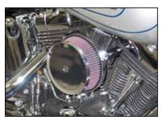
13. It will be necessary for all K&N<sup>®</sup> custom air cleaners to be checked periodically for realignment, clearance and tightening of all connections. Failure to follow the above instructions or proper maintenance may void warranty.
