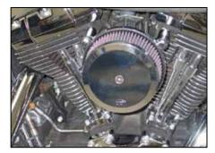
12. Install the filter cover plate onto the K&N<sup>®</sup> air filter and secure with the provided hardware. **NOTE: Be sure to place one drop of thread locker to the cover plate mounting bolt.**
