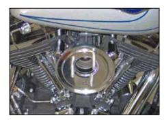
9. Install the three spacer/bolts into the K&N<sup>®</sup> filter base plate, then install the base plate gasket and one drop of thread locker onto each spacer/bolt. Install the K&N<sup>®</sup> filter base plate assembly onto the breather plate as shown.
