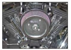
11. Install the K&N<sup>®</sup> air filter onto the base plate and secure with the provided hardware. **NOTE: Be sure to apply one drop of thread locker to each bolt.**
