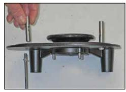
8. Install the two spacers onto the K&N® filter base plate with the provided hardware as shown NOTE: Place one drop of thread locker onto the threads of each bolts.
