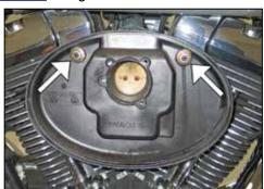
4. Remove the two crank case breather bolts shown.
