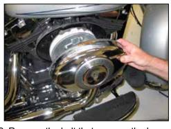
2. Remove the bolt that secures the bonnet to the filter assembly and then remove the bonnet from the vehicle.
