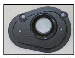
7. Install the venturi and three provided bolts into the K&N® filter base plate as shown.
