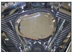
11. Set the top plate onto the K&N® air filter and install the filter assembly onto the vehicle, secure with the provided hardware.
