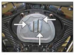
3. Remove the three bolts which secure the air filter to the filter base and then remove the <a href="mailto:air filter">air filter</a> along with the crankcase breather tubes.
