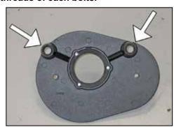
9. Install the two provided o-rings onto the  $K\&N^{\otimes}$  filter base plate as shown.
