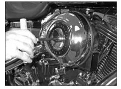
2. Remove the <u>air filter</u> cover mounting bolt and then remove the cover from the vehicle.
