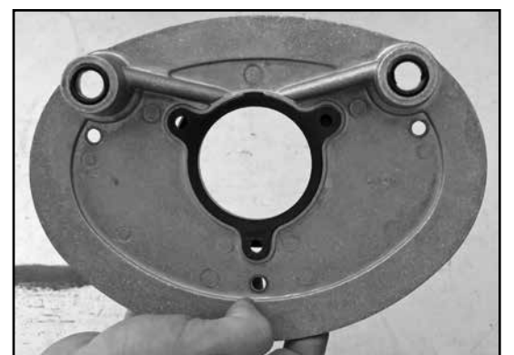
8. Align the holes on the velocity stack with the bolt holes in the back plate.
