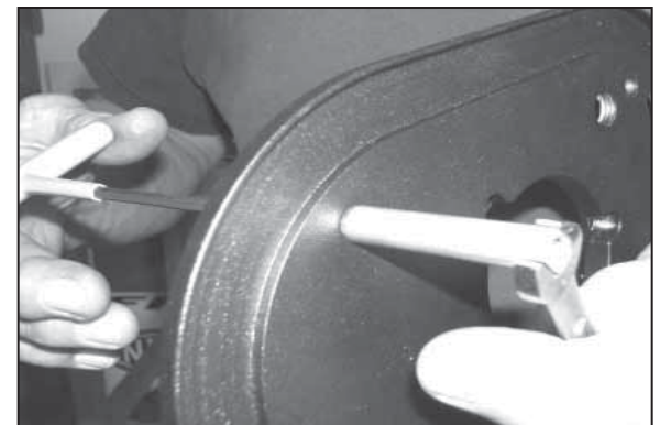
8. Install the four bolts from step 8 through the back plate and thread the bolts into the provided spacers.
