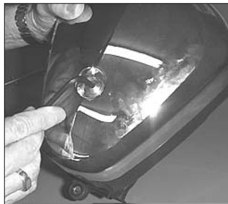
5. Remove the center bolt from the outer cover and remove the cover.
