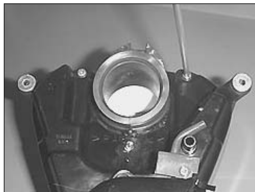
4. Remove the two screws from the back of the air box.
