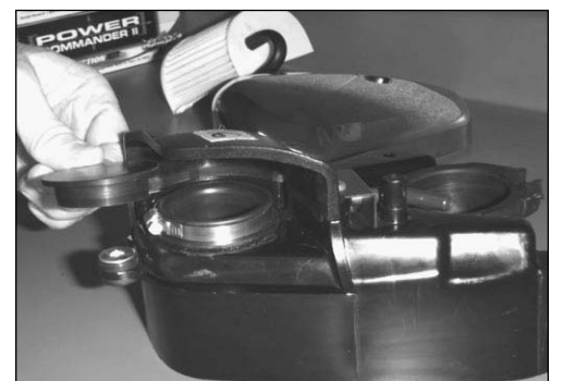
9. On the 1999-2003 models install the supplied round intake plug. Securely tighten the hose clamp.
