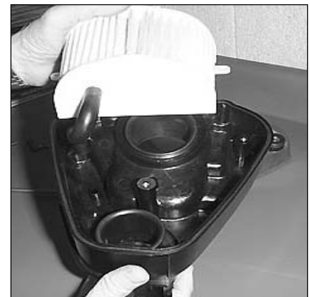
7. Remove the air filter and breather hose. Note: The breather hose will not be reinstalled.
