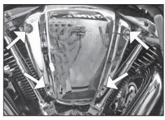
1. Remove the four socket bolts that hold the cover on and remove the cover.
