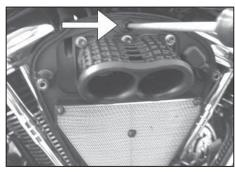
2. Remove the air filter screw.
