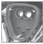
29. Install the K&N® air filter onto the backplate. NOTE: Make sure the air filter is completely seated onto the back plate.
