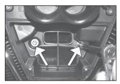
5. Remove the two lower air cleaner housing
