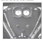
24. Hold the back plate to the throttle assembly. Install the five provided allen bolts and tighten. NOTE: It may be necessary to slightly move the velocity stacks. Make sure they are seated when you tighten the bolts.
