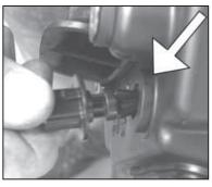
10. Remove the air temperature sensor from the air cleaner assembly.
