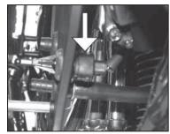
25. Plug the air temperature sensor wiring into the air temperature sensor.
