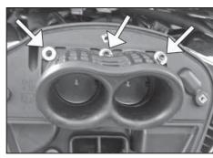
4. Remove the five duct bolts. NOTE: There are three on the top and two on the bottom.
