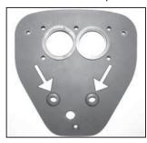
14. With the back of the back plate facing you install the two rounded grommets into the top left and top right holes.
