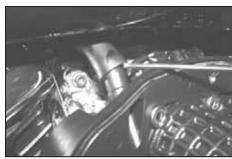
6. Disconnect the crankcase breather tube from the top of the air box.
