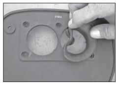
11. Install the supplied velocity stacks into the provided back plate.
