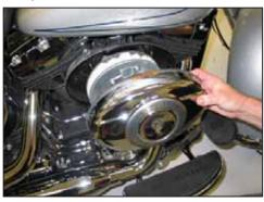
2. Remove the bolt that secures the bonnet to the filter assembly and remove the bonnet from the vehicle.
