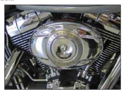
15. Install the filter bonnet onto the air filter and secure with the factory bolt.
