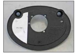
7. On models equipped with an EVAP vent line, cut out the provided template and place it on the filter base plate as shown. Mark the base plate for drilling a ½"ID hole.
