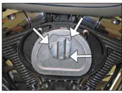
3. Remove the three bolts that secure the air filter to the filter base and remove the <u>air filter</u> along with the crank case breather tubes.
