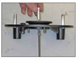
10. Install the three provided spacers onto the base plate as shown.
