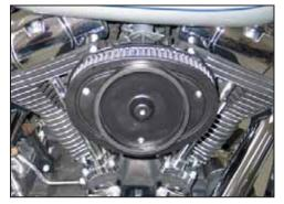
14. Install the air filter onto the base plate and secure with the three bolts provided.
