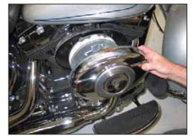
2. Remove the bolt that secures the bonnet to the filter assembly and then remove the bonnet from the vehicle.
