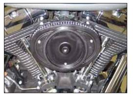
14. Install the air filter onto the base plate and secure with the provided three bolts. **NOTE: Apply one drop of thread locker to each bolt.**
