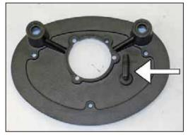
8. On models equipped with an EVAP vent line, drill a  $\frac{1}{2}$ "ID hole in the base plate at the location marked in step #7. Then install the provided grommet and 90° hose mender as shown.
