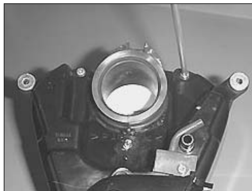
4. Remove the two screws from the back of the air box.
