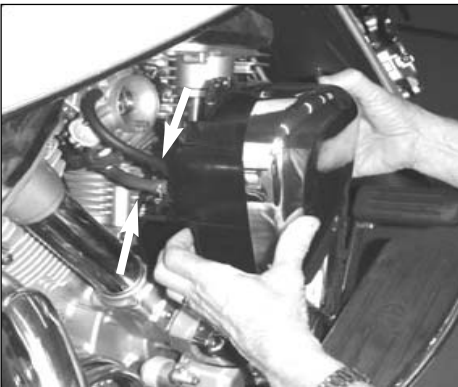
3. Remove the air cleaner housing and disconnect the two breather hoses from the rear of the housing.
