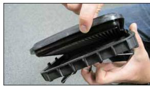
12. Remove the stock filter and Install the new K&N® filter.
