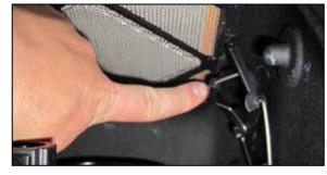
11. Pull bars down to release air filter cage & filter then wipe out any dirt or debris from the air box.
