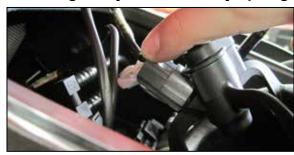
8. Disconnect front and rear injector connectors.
