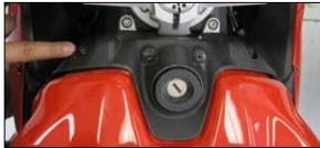
3. Remove the four allen screws shown and remove ignition cover above fuel tank.
