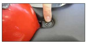
1. Loosen the allen screw shown and remove the seat.
