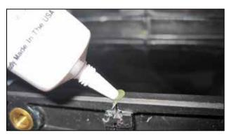
1. Using supplied grease; apply 2 separate beads of grease in the area shown.
