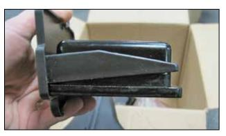
2. Insert filter into frame. Note the features on one side of the filter. These must go into the air box first during installation.
