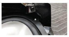
5. install the factory latch lever using the factory screw and supplied rubber grommet.
