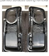
6. Install the supplied grilles to the lids using the supplied screws.
