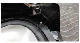
5. install the factory latch lever using the factory screw and supplied rubber grommet.
