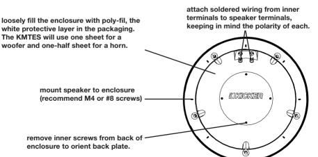
**Wiring:** Attach the wiring from your amplifier to the outer speaker terminals. Attach the included internal wiring from the KMTES to your speaker, and then mount the speaker to the enclosure. If you are using a speaker or grille equipped with LED wiring, run this wire through the LED wire port located underneath the outer speaker terminals and then through the LED wire grommet.
