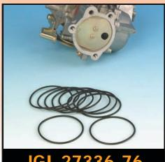
O-RING, CARBURETOR TO MANIFOLD
