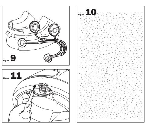
11. Using the included wooden tool, carefully push the wires into the gap between the helmet liner and shell. See Figure 11.
