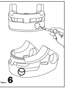
4. Mark an area in the nose section just to the left of center to mount the microphone. **See Figure 6.** Make sure that this placement will not interfere with any venting mechanisms or other parts of the helmet upon re-installation of the nose section.
