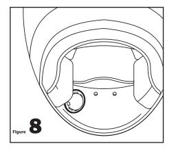
8. Reinstall the nose section and/or cheek pads & push the speakers and microphone firmly against the hook and loop fastener pads.
