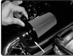
**19.** Tighten filter using 8mm nut driver.
