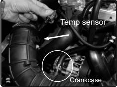
**7.** Carefully pull out the temperature sensor out of intake tube. With pliers, disconnect clamp on crankcase line and pull hose away from the fitting.
