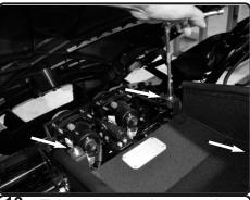
**13.** Tighten all nuts and screws using 10mm socket and ratchet.
