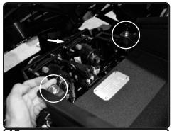
**12.** Secure the heat shield using provided M6 nuts and fender washers.
