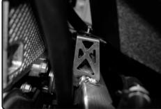
**11.** Now secure the back bracket to the factory air box mounting postion. Secure using provided m6 hex screw and fender washer.
