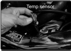
**21.** Install the temperature sensor into the grommet #6014.
