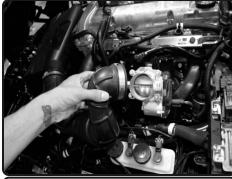
**3.** Now lift up and pull back the intake tube from the throttle body.
