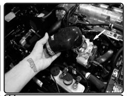
**14.** Install the cobra head to throttle body with clamps provided. Do not tighten clamps.
