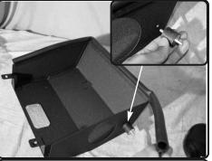
**6.** Install the provided rubber trim to the top of the heat shield. Notch corners for easy installation with pliers. Install the m6 vibramount to the thredded insert on heat shield.
