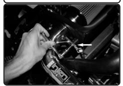
**20.** Tighten the vibramount using 10mm socket and ratchet.
