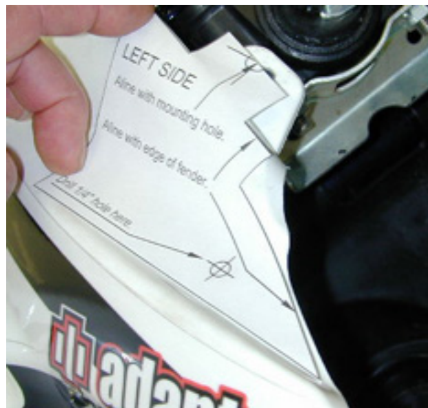
Drill template placement.
