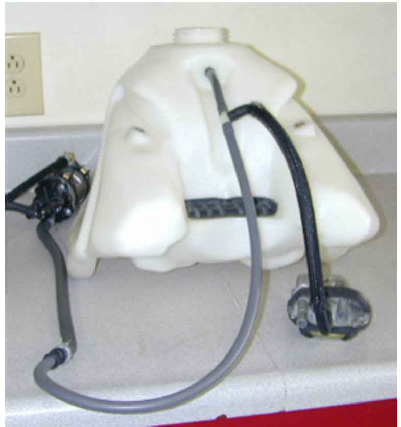
Fuel pump vent line routing
